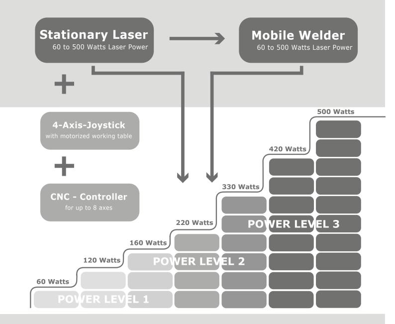
The key feature of our high-performance laser-welding systems is their modular design so that every device can be adapted to the specific requirements of the customer. The modular concept enables the systems to be used in a flexible manner for a broad range of applications. It also simplifies maintenance. Additionally, we offer special solutions for enhanced accessibility, automation and increase of power. Overview of options:
